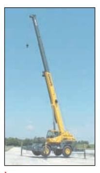
31 - 75 ft. (9.4 - 22.9 m) three section full power boom; maximum tip height: 84 ft. (25.6 m)
